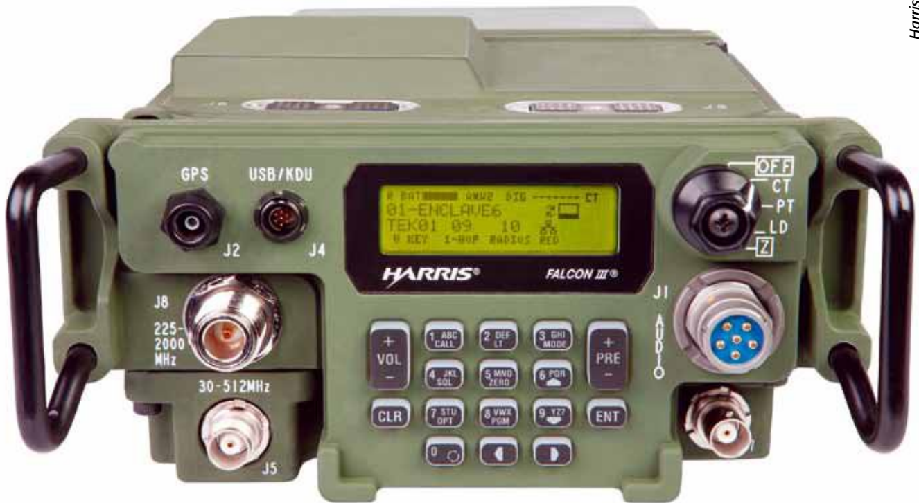
Harris' AN/PRC-117G radio has been enhanced with the wherewithal to accommodate the MUOS waveform to enable the transceiver to perform SATCOM.
